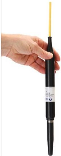
» The new architecture of the icListen Kayak has simplified arrays; With the new Universal Hydrophone Bus, or UHB, users can now string up to 100 hydrophones on a single cable, making it easy to design and deploy, large scalable arrays. (Photo credit: Ocean Sonics)
